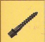
These are made from medium and low carbon steel by forging and thread rolling process. The shank diameter ranges from 16 mm to 25 mm. They are available in both black and galvanized condition
